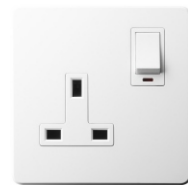
A5013SN 13A 250V~ 1 gang switched socket with Neon
