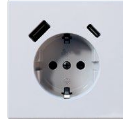
Schuko Socket with USB A+C 16AX 250V~2P+T USB 25W Item list
