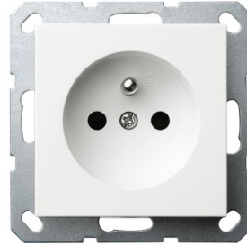
G5502 French socket with earth with children shutter protection 16A 250V~ 2P+T
